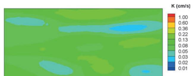
**Figure 3.**  $K$  distribution obtained through kriging of core scale  $K$  data from permeameter analysis.
